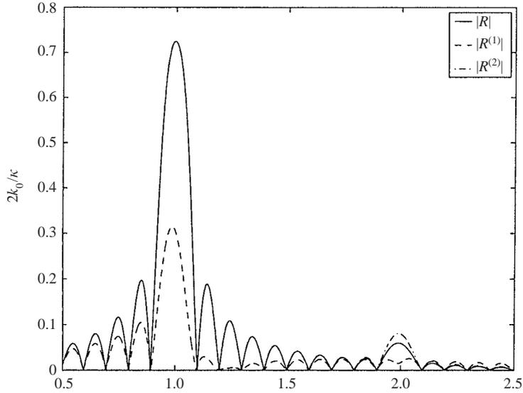
FIGURE 1. Comparison of the reflection coefficients for the periodic bedform described in the text.  $|R|$  corresponds to the modified mild-slope equation,  $|R^{(1)}|$  to the standard mild-slope equation and  $|R^{(2)}|$  to the revised mild-slope equation.
